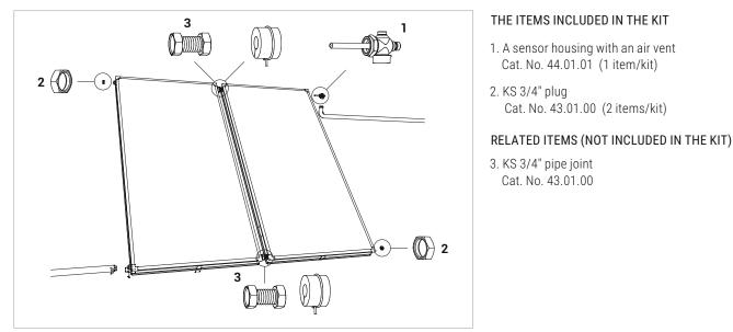
Note: There is only 1 x S19x1.8 O-ring included in the kit. Others are added to the solar collectors. The 3x3 O-ring installed in the sensor housing was pre-cut at the factory to facilitate installation.
